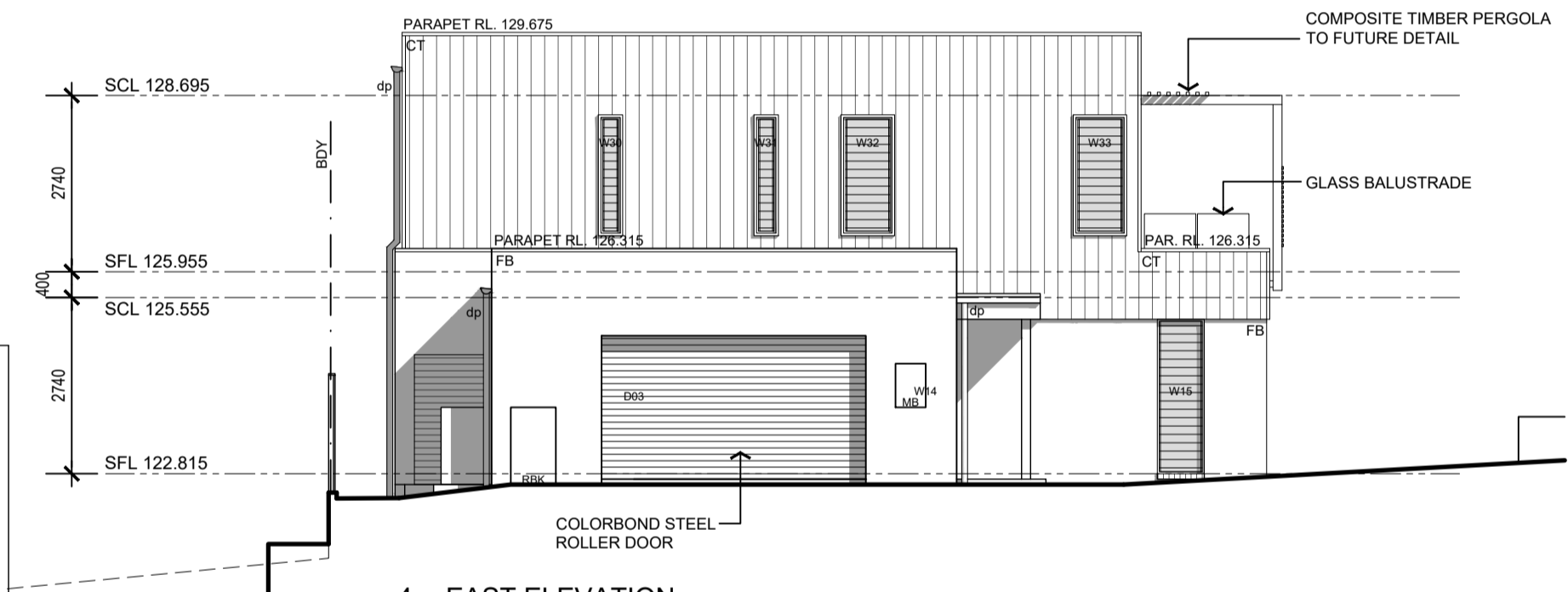
4 EAST ELEVATION Scale 1:100 (INCLUDES EAST ELEVATION OF 74 FINGAL AVE)
